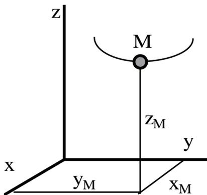
$$\left. \begin{aligned} x_M &= x_M(t) \\ y_M &= y_M(t) \\ z_M &= z_M(t) \end{aligned} \right\} \text{– закон движения точки;}$$
